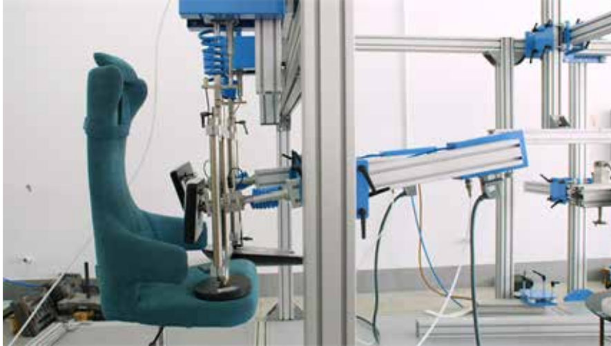
Figure 5.2.14 Office chair being mechanically tested
