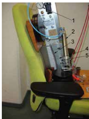
Figure 5.2.27 Lumbar support protrusion and height measurement (overall view)
