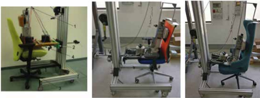
Figure 5.2.25 Examples of CMD placement fixture with chair and CMD
