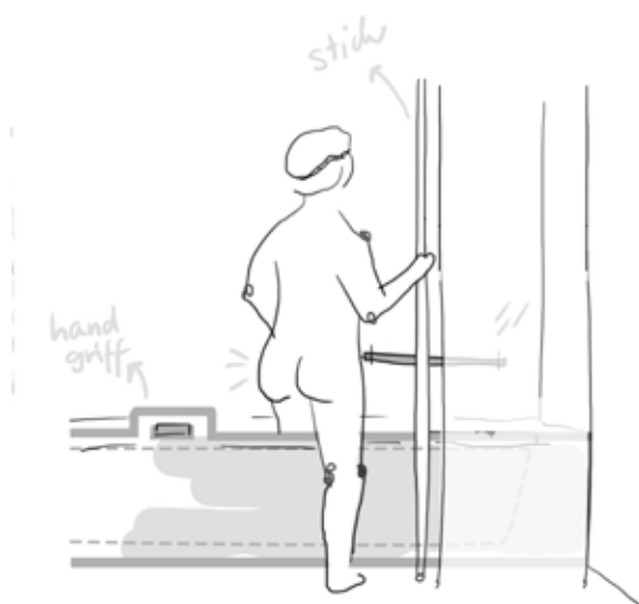
Figure 4.1.24 Ensuring safety in the bathroom by using rails and handles supports also socialization thus it is easier to maintain hygienic standards in personal hygiene and maintenance of housing spaces that are connected also with bigger self/confidence by interaction with other people in public spaces and at home as well (Valábeková, Kira)
