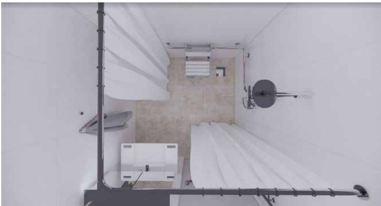
Figure 4.1.35 Railing with drawing/sliding curtain is the best solution for an adaptable shower, the disadvantage is more water sprinkled in the room; bathrooms for the DSS Rača, (Tomová)
