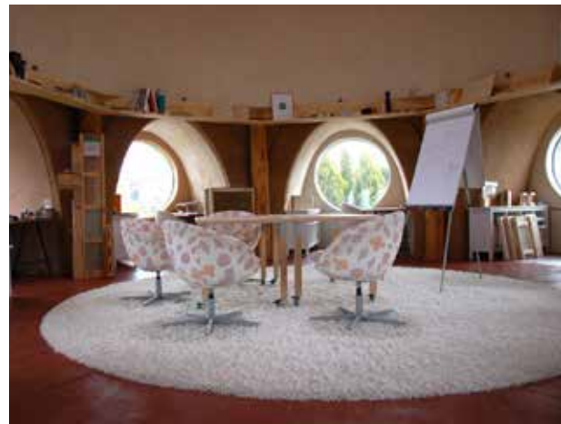
Figure 4.3.10 Self-bearing Straw bale dome made in passive standard, in Hrubý Šúr, Slovakia, is the headquarter of the architecture studio Createrra, made of natural renewable materials: straw bales as the main construction material, wood structure, with using of green roof on the top, clay floor finished with flax oil varnish, walls covered by clay plaster (Createrra)
