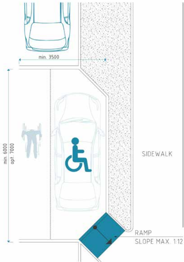
Figure 3.3.23 Parking space dimensions in longitudinal parking layout (Čerešňová, Suláková)
