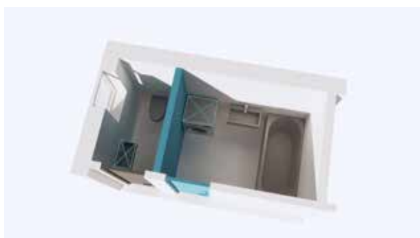
Figure 3.3.6 a, b, c, d Accessible bathroom is achieved by removing the wall between the bathroom and the toilet. No plumbing and pipe fittings can be installed on the removable wall. The bathroom floor must be sloping into the floor drain (Rollová, Suláková)
