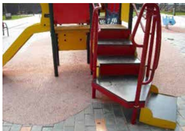
Figure 3.3.19 a, b Accessible elevated play equipment with transfer system – transfer steps and platform by HAGS, Sweden (Čerešňová)
