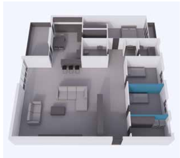
Figure 3.4.1 Adaptable apartment and removable walls that allow changes in the number or size of rooms (Rollová, Suláková)
