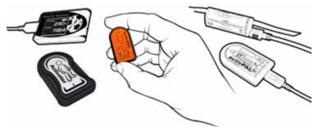
Figure 2.3.8 Devices for measuring the physical activity via accelerations of the body segments
